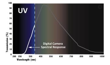
When it comes to ultraviolet (UV) imaging, it's important to distinguish between UV light and UV-fluorescence imaging. Although they both use UV lighting, they're entirely different. UV imaging starts with passing the emission of a UV-emitting LED, lamp or diode, or looking at a subject illuminated with UV light that's reflected off the item being inspected. The reflected UV light is then captured by the camera. The wavelength of the UV light is not converted or shifted in this process.
