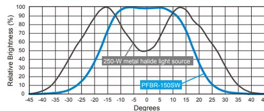
\* Actual measurement values with intensity of 100%, a bundle of Ø8 mm, a straight light guide with a total length of 1,100 mm installed, and at a position 600 mm away from the fiber output edge. (Results may vary for individual units.)
