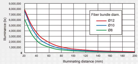
\* Actual measurement values with intensity of 100%, bundles of  $\varnothing 8$ , 10, and 12 mm, a straight light guide with a total length of 1,080 mm installed, and at positions at each illuminating distance away from the fiber output edge. (Results may vary for individual units.)
