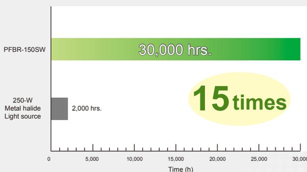
\* Calculated values up to intensity of 100%, ambient temperature of 25 °C, and light output drop up to 70%. (Results may vary for individual units.)
