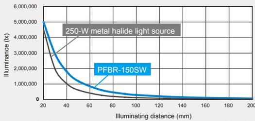
\* Actual measurement values with intensity of 100%, a bundle of  $\varnothing 8$  mm, a straight light guide with a total length of 1,100 mm installed, and at positions at each illuminating distance away from the fiber output edge. (Results may vary for individual units.)
