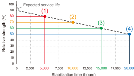
Relationship between Light Quantity Feedback Control Function and Stabilization Time (Representative)
